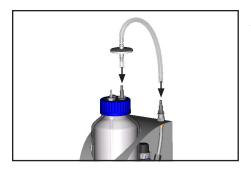
Assemble tubing with filter.
