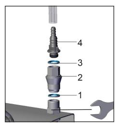
Assemble coupling (2) with seals (1, 3) and hose nozzle (4).
