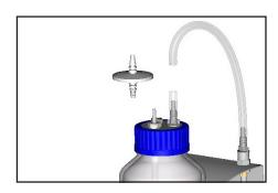
Remove connecting tube from the filter. Remove the filter from the piece of tube at the hose nozzle.
