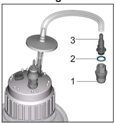
Assemble coupling part (1) with seal (2) and hose nozzle (3).
