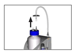
Remove the connecting tube from the filter, isolate connections in case.
