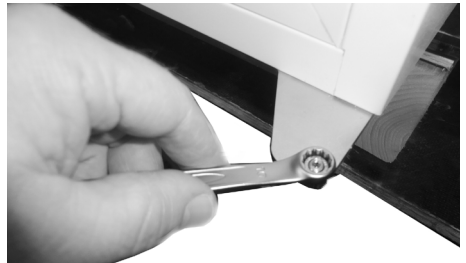
24. Remount and tighten pivot nut
