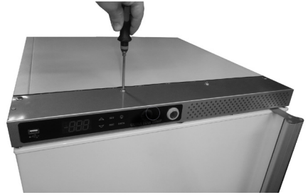
44. Remount the four top screws
