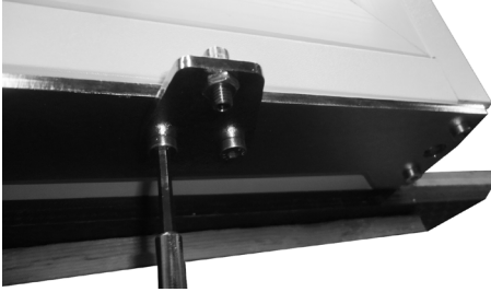
19. Remove bottom handlelock pin plate by loosening two screws (use 4 mm allen key)
