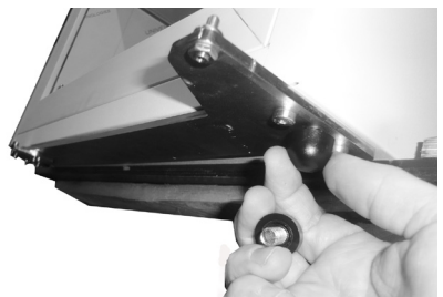
18. Remove the two front feet
