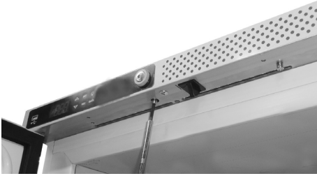
43. Remount the lock pin
