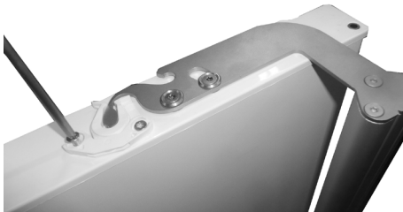
31. Go to the current door bottom and de-mount two screws from the door closer (use Torx 20 tool)
