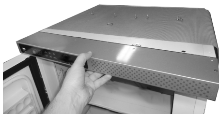
40. Carefully push the toppanel back into position
