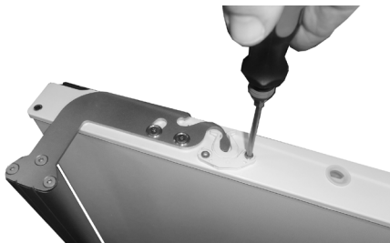
37. Remount the two screws and the door closer is fixed
