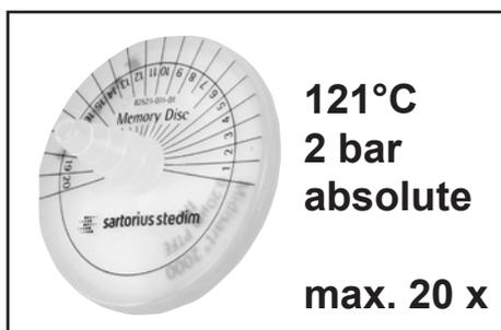
The number of autoclaving cycles can be marked on the plastic disc (Memory Disc) of the filter (max. 20 autoclaving cycles according to the manufacturer instruction).
