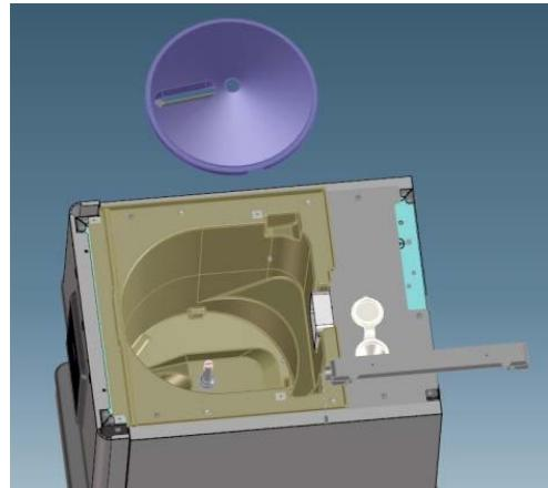
7. Using the same carafe, prepare again 500 ml of warm water (40-50°C) and 15 ml of Scotsman Sanitizing product and pour of the solution on the internal sides of the storage bin
