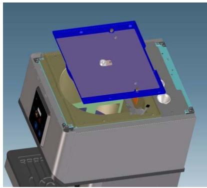
10. Remove, clean and reinstall the air filter located on the right side panel, then open the water tap
