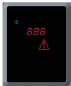
Hold the red capacitive alarm button pressed for five seconds to display the current alarm, then refer to the following table listing the suggested solutions; in any case also inform the Scotsman service centre.
