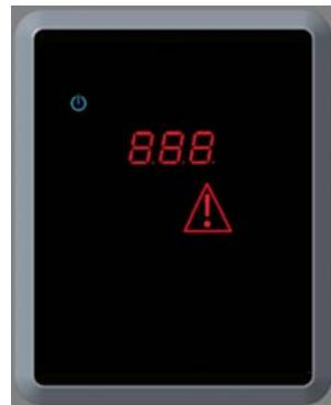
Press the button for 5 seconds to display the current alarm.
