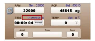
When remove the shift running conditions, select MENU-Program-Program CALL and press the 'Shift'part to:delete Press 'Clear all' button at the setting window of shift running to delete all steps.
