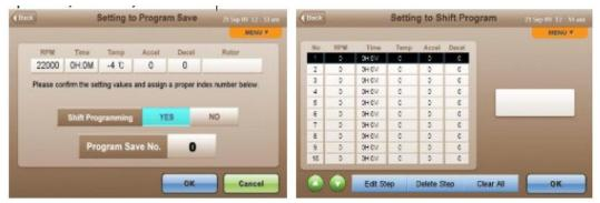
Press 'OK' button to complete setting. The 'shift' program is displayed on the main: operational screen as '1/1:0H:0M:0S:(S)' on the top of TIME display.
