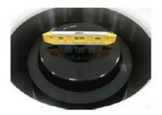
Mount the rotor and place the magnetic precision level on the middle of a rotor.
