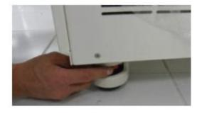
To adjust the balanced position, rotate the red colored ring at the wheel caster counterclockwise until well balanced. This adjustment of rubber leg also fixes the instrument by holding the wheel caster.
