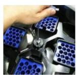
3-6-4. To open or close of rotor lid, grasp the rotor with one hand and rotate the rotor lid nut counterclockwise for opening, and clockwise for closing. Or the rotor lid open/close tool can be used as follows.
