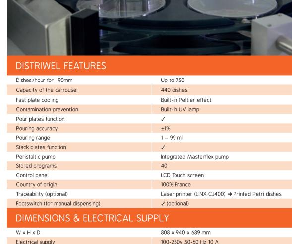
100-250v 50-60 Hz 10 A Electrical supply 150 W
